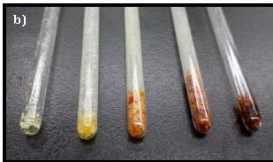
Figure 3-13. Color development for samples of Linseed Oil aged with (a) UV light (centered at 254 nm, 15 W) and (b) Heat (90 to 210°C).
