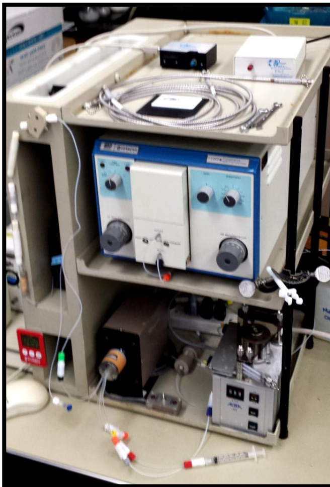
Figure 2-9. Photograph of the RP-LC system.
